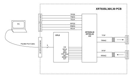
Figure 1 Simplified Block Diagram of the XRT83SL30/L30EVAL Application Board
