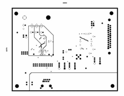
Figure 10 XRT83SL30/L30EVAL Layout Plot-Power Plane
