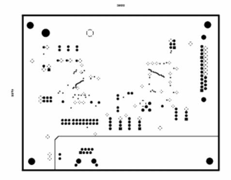
Figure 9 XRT83SL30/L30EVAL Layout Plot-Ground Plane
