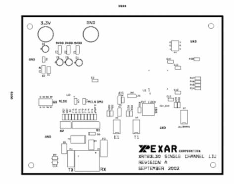
Figure 7 XRT83SL30/L30EVAL Layout Plot-Top Silk Screen
