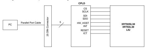
Figure 2 Simplified Block Diagram of the CPLD Interface
